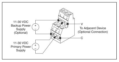
Figure 2-7. FBUS-HSE/H1 Power Connector Pinout
